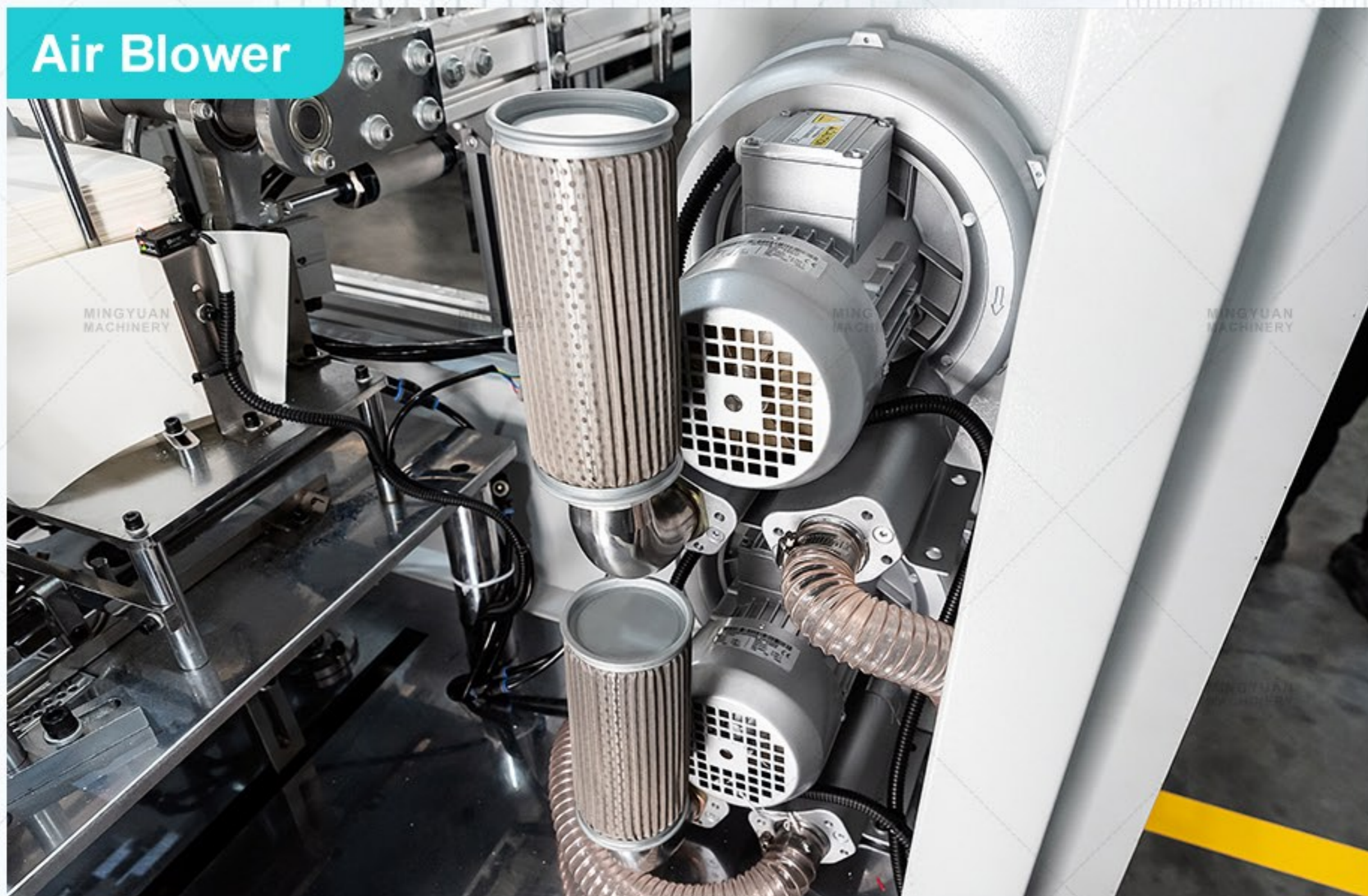
Supply of air continuously to the hot air heater.
