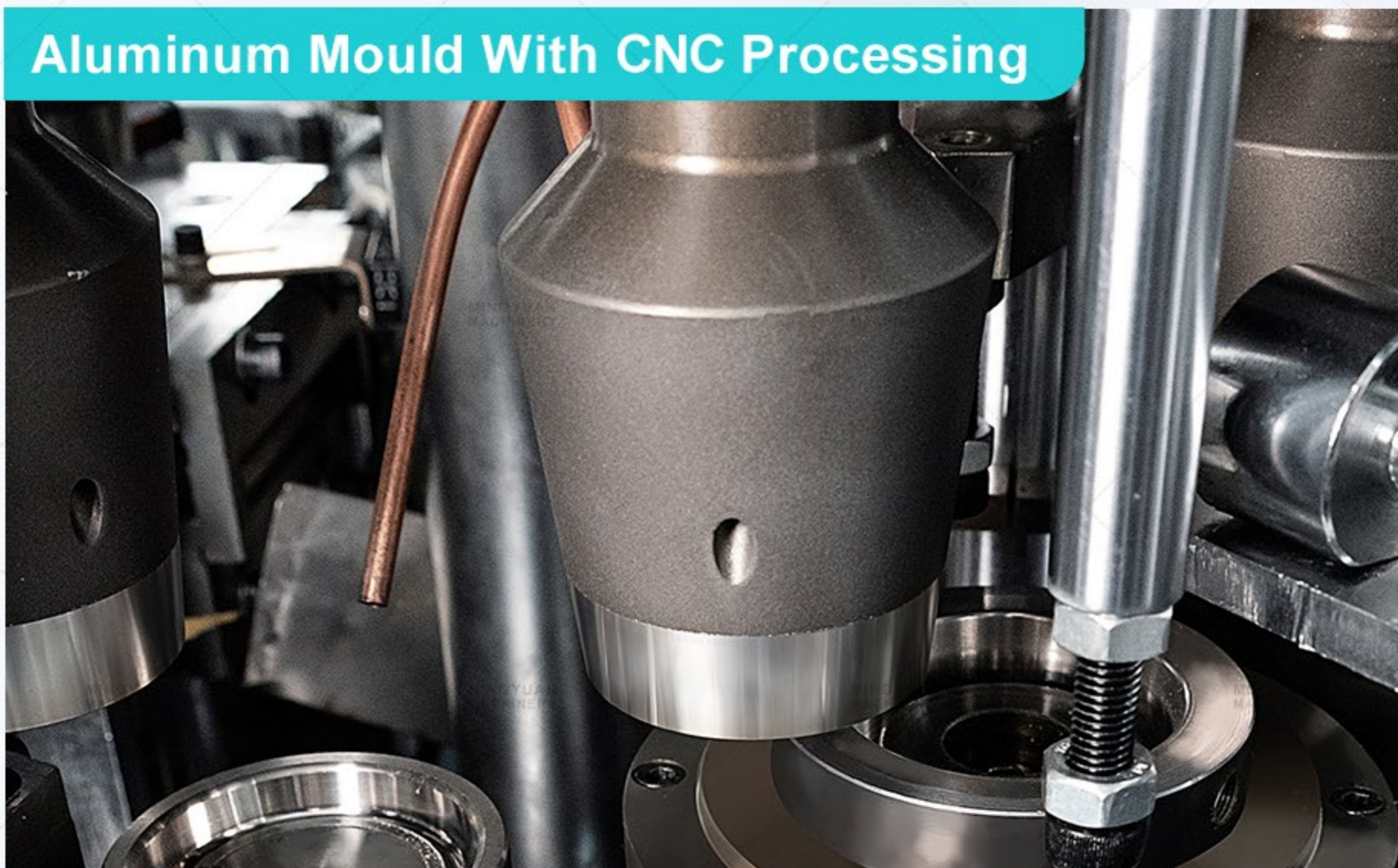
It is best choice for high speed machine compared with the iron mould, lighter in weight, greatly improves the torque force of the spindle, longer service life and better quality.
